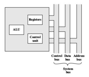
The ALU does the actual computation or processing of data. The control unit controls the movement of data and instructions into and out of the processor and controls the operation of the ALU. In addition, the figure shows a minimal internal memory, consisting of a set of storage locations, called registers.
