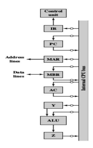
A single internal bus connects the ALU and all processor registers. Gates and control signals are provided for movement of data onto and off the bus from each register. Additional control signals control data transfer to and from the system (external) bus and the operation of the ALU.
