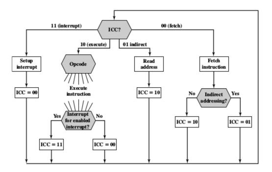
We assume a new 2-bit register called the instruction cycle code (ICC). The ICC designates the state of the processor in terms of which portion of the cycle it is in:
